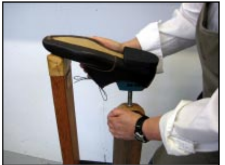
Step 4 : Rest the toe of the last on the leather pad and release the spring loaded post. Adjust for a snug fit.
