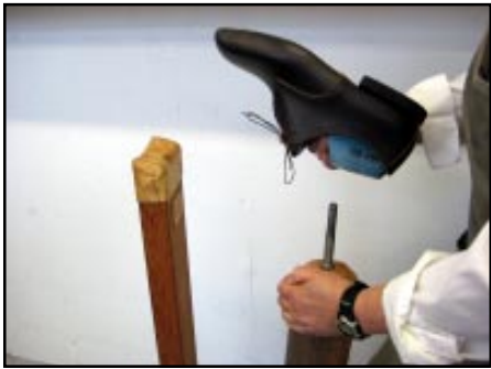
Step 2 : Align the "Adjustable Pin" with the thimble in the heel of the last.
