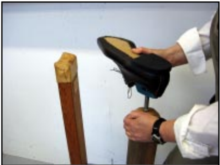
Step 3 : Place the "Adjustable Pin" into the thimble of the last. Be sure the last goes all the way down on pin.
